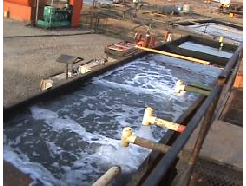
Simple tank and chemical produced water treatment system used in Colombia that processed over 10 million bbls
