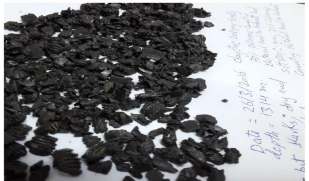
Figure 2: Depth 1314m; Inclination 28°; Kolosh T3. MW 11.5ppg of Silicate Mud. Bit marks clearly visible, a mark of cuttings integrity
