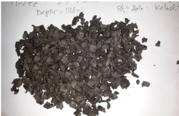
Figure 1: Depth 1108m, Inclination 15°; Kolosh T1.MW 11.0 ppg; Silicate Mud. Bit marks clearly visible, a mark of cuttings integrity.
